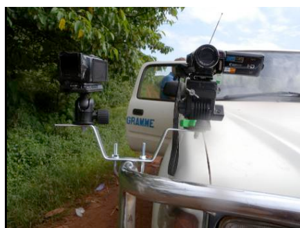
Figure 5-15: Cameras Mounted on the Guard Rails of the Vehicle
