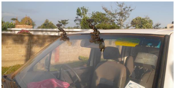
Figure 5-19: ContourGPS Camera Clamped on the Vehicle Windscreen
