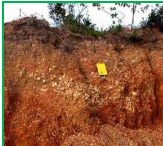
Variability of in situ natural hill-gravel (colluvium)
