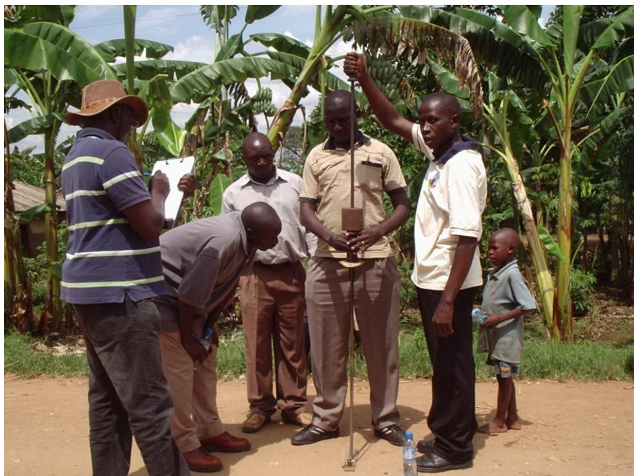
Figure-5: Busamaga – Magada In-situ Strength determination using the Dynamic Cone Penetrometer.
