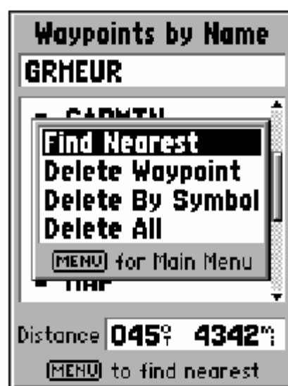
Figure-7: Deleting waypoint – "Menu" Key twice → "Points" menu → "Menu key" → "Delete All" command
