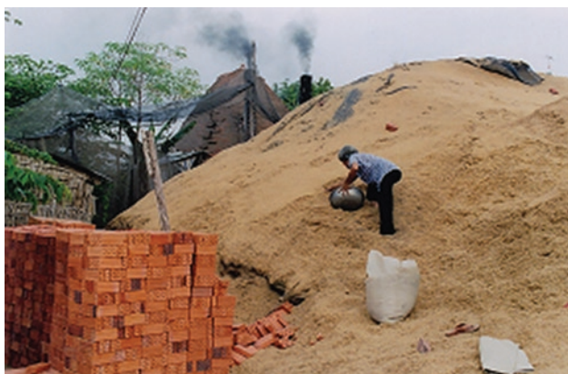
Photo 7: Clay Brick production using rice husk fuel
