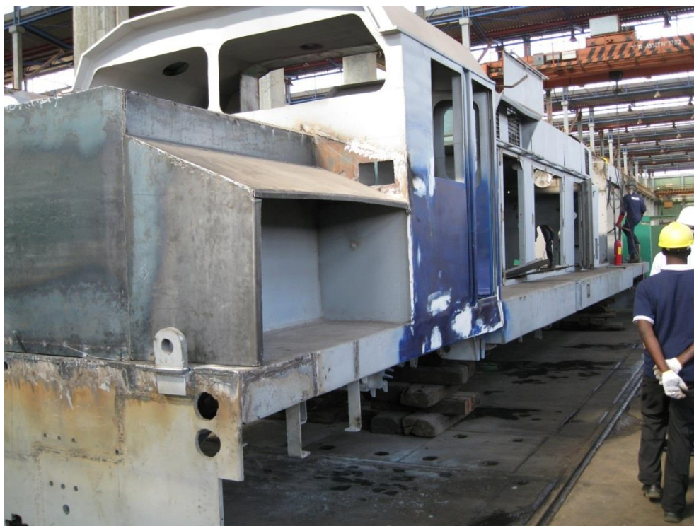
Figure 45 Re-manufacturing of main line 88xx class Canadian Diesel Electric locomotives at the Morogoro locomotive workshop
